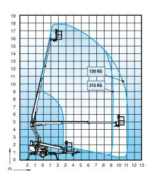
Max. working height 18.00 m Max. platform height 16.00 m 11.20 m Max. outreach Support width 3.9/4.3 m Lifting capacity 215 kg Basket size 0.70 x 1.30 m Boom rotation cont. Basket rotation 180° Boom control proport. 6.70 m Transport length Transport width 1.95 m 2.29 m Transport height Weight 2300 kg Driving system std AC-socket in the basket x 2 std Electro motor std Petrol power pack opt. Diesel power pack opt. Gradeability 25%
