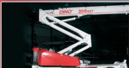
Long outreach with stable articulated boom – for 'up and over' access, with telescopic top boom section.
