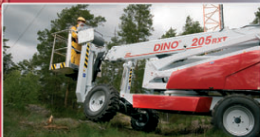
Oscillating front axle – ensures that all the wheels are in contact with the ground, giving maximum traction.
