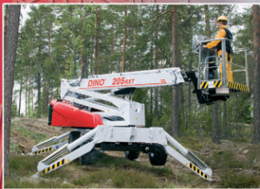
Hydraulic outriggers with impressive levelling ability – the platform can be operated on severely sloping terrain.
