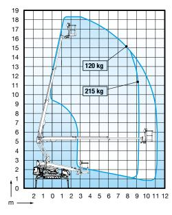
Max. working height 18.50 m Max. platform height 16.50 m Max. outreach 11.20 m Support width 3.54 / 3.95 m 215 kg Lifting capacity Basket size 0.7 x 1.3 m Boom rotation cont. Basket rotation 180° Boom control proport. Transport length 5.93 m Transport width 1.40 m / 1.18 m Transport height 1.98 m Weight 2860 kg AC socket in the basket x 2 Diesel engine std, Kubota 17.3 kW Length of tracks 1.93 m
