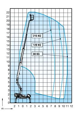
Max. working height 22.10 m Max. platform height 20.10 m Max. outreach 11.00 m Support width 3.54 / 3.95 m Lifting capacity 215 kg Basket size 0.7 x 1.3 m Boom rotation cont. Basket rotation 180° Boom control proport. Transport length 6.30 m Transport width 1.40 m / 1.18 m Transport height 1.98 m 3060 kg Weight AC socket in the basket x 2 std Diesel engine Length of tracks 1.93 m Gradeability 43 %
